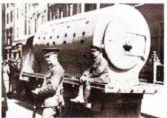
vehicle was made by bolting four boilers onto the rear of a Guinness's
